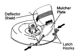
ACAUTION: Do not remove deflector shield from mower. Raise and hold shield when attaching mulcher plate and allow it to rest on plate while in operation.
