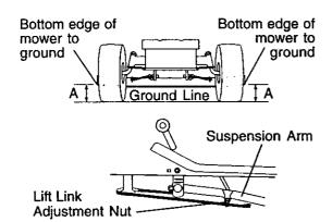
FRONT-TO-BACK ADJUSTMENT IMPORTANT: Deck must be level side-to side. If the following front-to-back adjustment is necessary, be sure to adjust both front links equally so mower will stay level side-to-side.
