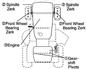
**①SAE 30 or 10w30 MOTOR OIL @GENERAL PURPOSE GREASE ③REFER TO Maintenance "ENGINE" SECTION**
