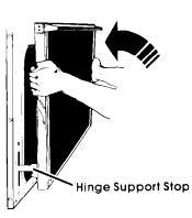
2. Hold the door on both sides and lift slightly to clear the stops in the hinge supports.
