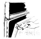
5. During broiling the oven door must be partly open. A built-in stop will hold it there.
