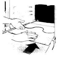
Slide the foil under the bake element.
