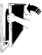
2. Lift slightly while sliding the hinge supports into the openings.
