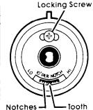
2. Loosen the locking screw; NOTICE position of notches.
