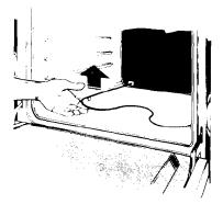
Lift **the cool bake element** slightly to lift the feet off the oven bottom.
