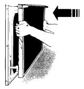
3. When the stops in the hinge supports slide into the oven openings, the door will snap into place and can be closed.
