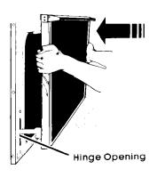
1. Fit the hinge supports into the openings at the bottom oven corners.
