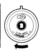
To lower the temperature, move black part of knob closer to LO. Each notch equals about 10 F (5 C).
