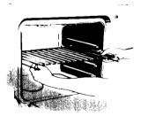
Lift rack at front and pull out.
