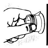
1. Pull the Oven Temperature Control straight off.
