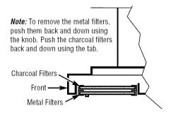
For proper operation, be sure to use the charcoal filters in the upper set of filter holders and metal filters in the lower set of filter holders.
