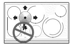
Sliding aluminum or copper clad bottom pans on the cooktop can cause metal markings on the cooktop surface. These marks should be removed **immediately** after the cooktop has cooled using the cooktop cleaning cream. Metal marks can become permanent if not removed prior to future use.
