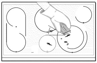
If soils remain, carefully scrape soils with a metal razor blade scraper, holding scraper at a 30 degree angle to the surface. Remove loosened soils with cooktop cleaning cream and buff surface clean.
