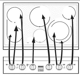
Location of the Radiant Surface Elements and Controls Figure 1
