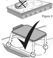
Figure 6 - Make sure the feet of the griddle are not directly on the burners.
