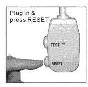
The power supply cord contains a current device that senses damage to the power cord. To test your power supply cord do the following:
