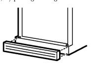
**4.2** Move the bottom hinge bracket (and shim glued to it) and plastic washer from the right side to the left side.
