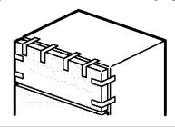
**2.2** With a 5/16" hex-head socket driver, remove the screws that hold the top hinge to the cabinet.
