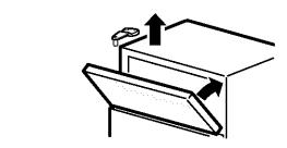
**6.2.3.** Make sure the door is slightly above the top of the cabinet and the gap between the doors is even across the front. Tighten the top hinge screws. Do not overtighten these screws—tighten them until they are just snug, then turn them another one-half turn.
