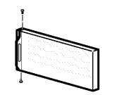
**5.4.3** Remove the screw from the right top edge of the door and insert it into the handle screw hole on the left side.
