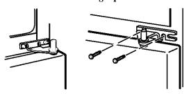
**3.3** Remove the tape and tilt the door away from the cabinet. Lift the door from the pin in the bottom hinge bracket. (If the plastic washer sticks to the door bottom, put it back on the hinge.)
