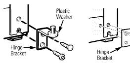
Models with a hinge bracket that has 2 screw holes.
