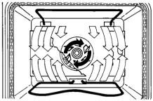
CONVECTION BAKE – The bottom element and outer top element operate at full power and glow red whenever heating. Air in the oven cavity is circulated by the fan for even heating and faster cooking. Use this setting for baking and roasting.
