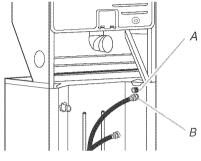
A. Cold water inlet valve (blue) B. Hot water inlet valve (red)
