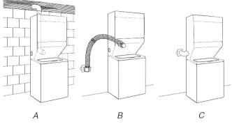
A. Standard rear offset exhaust installation
