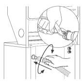
5. Place clamp over the area marked "CLAMP." Release clamp.
