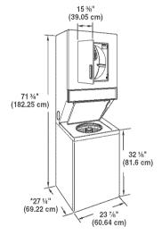
\*Most installations require a minimum 5½" (14 cm) clearance behind the dryer for the exhaust vent with elbow. See "Venting Requirements."
