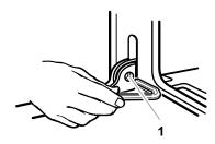
1. Insert small end of pin here
