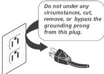
Power supply cord with 3-prong grounding plug CORRECT Use this way ONLY
