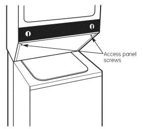
To ensure the Laundry Center is level and solid on all four legs, tilt the Laundry Center forward so the rear legs are off the floor. Gently set the Laundry Center back down to allow the rear legs to self-adjust. Place a level on top of the washer. Check it side to side, then front to back. Screw the front leveling legs up or down to ensure the Laundry Center is resting solidly on all four legs (no rocking of the Laundry Center should occur).
