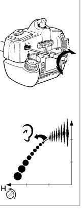
Therefore dismantle the cutting equipment, nut, support flange and disc drive before adjusting the high speed needle. The high speed needle is adjusted correctly when the machine 'splatters' a little . If the machine smokes heavily at the same time as it 'splatters' heavily the adjustment is too rich.
