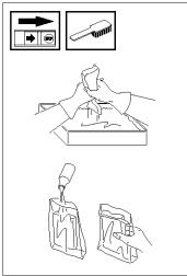
the filter on the machine. Never use common engine oil. This would drain through the filter quite quickly and collect in the bottom.
