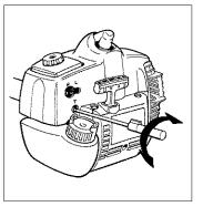
CAUTION! Contact your servicing dealer, if the idle speed setting cannot be adjusted so that the cutting attachment stops. Do not use the machine until it has been properly adjusted or repaired.
