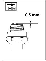
If the machine is low on power, difficult to start or runs poorly while idling always check the spark plug first. If the spark plug is dirty, clean it and at the same time check that the electrode gap is 0.5 mm. The spark plug should be changed after about one month of operation or earlier if necessary.
