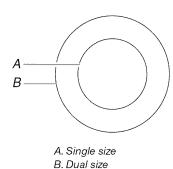
The dual size elements offer flexibility to cook using different sizes of cookware. The single element can be used in the same way as a regular element. The dual element combines both the inner and outer elements and is recommended for larger cookware.
