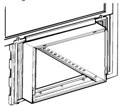
**NOTE:** Do not shut the window so tightly that movement of the accordion panels is restricted.
