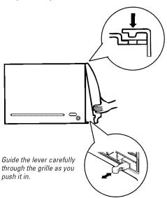
Lift the inlet grille and secure the front frame with a type A screw through the front grille. Lower the inlet grille back into place.
