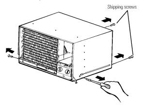
Slide the air conditioner from the case by gripping the base pan handle and pulling forward while bracing the case.
