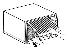
Clean the filter with warm, soapy water. Rinse and let the filter dry before replacing it.
