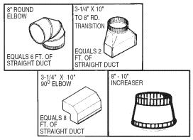
The system will operate most efficiently when the ductwork does not exceed 40 feet of equivalent duct. The illustrations, above, shows equivalent feet of elbows and transitions. The number of feet of straight duct plus the equivalent feet of transitions and/or elbows to be used should equal 40 feet or less.
