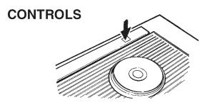
Turn the downdraft blower ON by pressing down on the activating switch. The air vent will rise.
