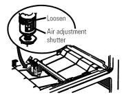
The shutter for the bottom (oven) burner is near the back wall behind the warming drawer, storage drawer or kick panel. Remove the drawer or panel. See the *Care and cleaning of the range* section.
