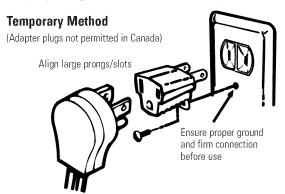
**ACAUTION:** Attaching the adapter ground terminal to the wall receptacle cover screw does not ground the appliance unless the cover screw is metal, and not insulated, and the wall receptacle is grounded through the house wiring. The customer should have the circuit checked by a qualified electrician to make sure the receptacle is properly grounded.
