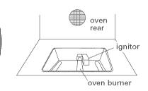
**26.** If the oven flame needs to be adjusted, locate the air shutter near the center rear of range. Loosen the locking screw and rotate the air shutter until the proper flame appears. Tighten locking screw.
