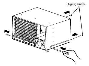
Slide the air conditioner from the case by C gripping the base pan handle and pulling forward while bracing the case.
