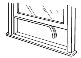
Carefully insert the plastic frame guides into B the bottom of the case on each side.
