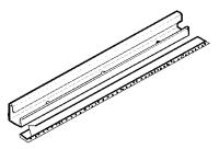
Install the top mounting rail with 3 type A D screws on the inside of the case. Insert the frames for the accordion panels into the top mounting rail and the frame guides. Attach the accordion panels to the side of the case using 5 type A screws.
