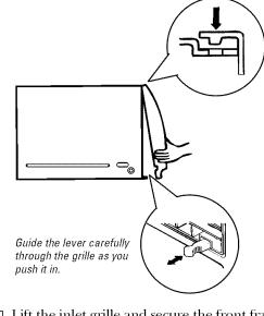
**D** Lift the inlet grille and secure the front frame with a type A screw. Lower the inlet grille into place.
