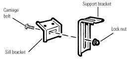
**B** Open the window and mark the centerline of the window stool. Measure and mark 11" to the left and right of the centerline.
