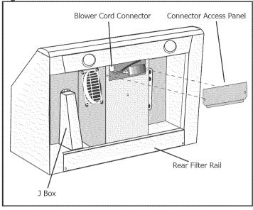
Figure 2 - DAH95 models with internal blower
