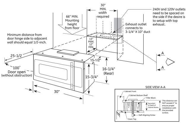
Note: Outside venting is optional. Vent (duct) can be horizontal or vertical.
