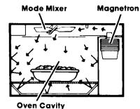
A magnetron in the microwave oven produces microwaves. The microwaves move into the oven where they are scattered or stirred by a mode mixer (like a fan). Microwaves bounce off metal oven walls and are
