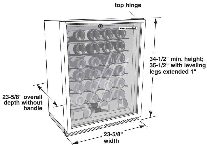
To ensure proper ventilation for your wine cellar, allow for a 1/4" (6.35 mm) space on each side and at the top. When installing your wine cellar next to a fixed wall, leave 2-1/2" (6.35 cm) minimum clearance on each side to allow for the door to swing open.
