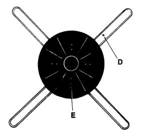
The removable filter continuously filters the wash water and traps the food particles that have been removed from the dishes on the outside of the filter. These trapped food particles are removed from the filter by the jet spray action of water from the single spray nozzle (D) underneath the wash arm. The ultrafine filter is cleaned by the nine water jets (E) underneath the 4-Way Hydro Sweep Wash Arm.
