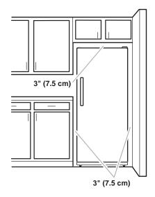
Allow at least 3 in. (7.5 cm) of air space at the top and on both sides of the refrigerator and 1 in. (2.5 cm) between the back of the refrigerator and the wall. If the refrigerator is to be against a wall, leave extra space on the hinge side so the door can open wider.
