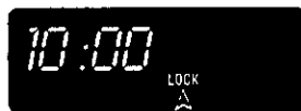
LOCK IS STILL ENGAGED. DOOR CANNOT BE OPENED UNTIL LOCK IS NO LONGER DISPLAYED.
