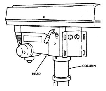
2. Using a 5mm HEX "L" wrench, tighten the two head lock set screws on the right side of the head.
