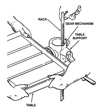
While holding rack and table support in an engaged position slide both down over column. Slide rack down column until rack is positioned against lower column support.
