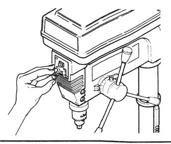
To turn drill ON, insert finger under switch lever and pull end of the lever out.
