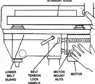
4. Loosen Belt Tension handle by turning clockwise.
