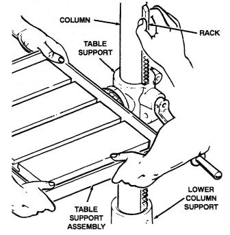
6. Replace column collar (bevel side down) and position it over rack. Tighten set screw in collar with 3mm HEX "L" wrench. Rotational position of set screw is not important. Collar must sit loosely over rack and must not be angled on the column. Only tighten set screw enough to keep collar in place; rack should still slide freely in collar when the table is swung to the left or right around the column.
