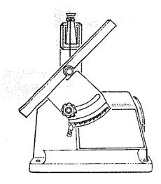
2. A bevel scale is provided under the work table as a convenient reference for setting the approximate table angle for bevel cutting.
