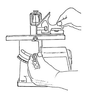
4. Loosen the screw holding the bevel scale pointer and adjust to  $0^{\circ}$ . Tighten screw.
