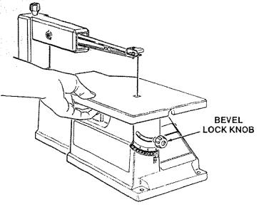
2. Use a small square to set the table at 90° to the blade. If there is too much space between the square and the blade, the table must be adjusted.
