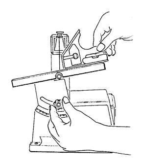
3. When the space between the square and the blade is minimal, tighten the bevel lock knob. The table should now be approximately 90° to the blade.
