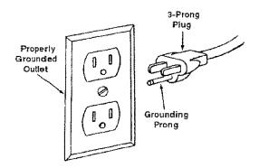
WARNING: Do not permit fingers to touch the terminals of plug when installing or removing the plug to or from the outlet.
