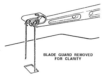
4. Locate the blade guard and carefully install it onto the saw as shown.
