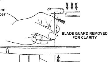
3. Look at the blade holders closely and notice the blade slots and pin recesses in the blade holder. The blade holder is made so you can position the blade for cutting from the front or one side of the saw.
