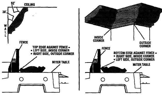
**CROWN MOLDING FLAT ON MITER TABLE**
