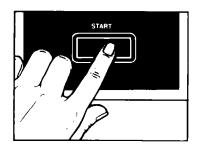
**4.** Push the START Button. The oven light will come on and cooking will begin. You will hear the fan running during oven operation.
