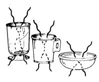
Microwaves pass through glass, paper and plastic without heating them so food absorbs the energy. Microwaves bounce off metal pans so food does not absorb the energy
