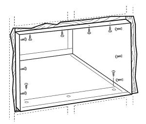
Place the case in the wall opening and secure with 12 1" long #10 wood screws.
