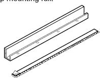
B Install the top mounting rail with 4 type A or 5 type A screws (as the installation requires) from the outside of the case.
