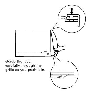
D Secure the front grille to the case by replacing the screw removed in Step 3. If a screw was not removed in Step 3, secure the grille with a type A screw for models with a raise-up inlet grille or a type D screw for models with a slide-out filter.
