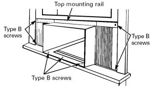
Extend the left and right accordion panels to the vertical window sashes and attach with 4 type B screws.
