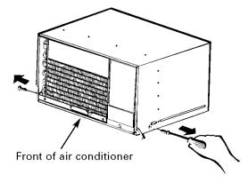
B Slide the air conditioner from the case by gripping the base pan handle and pulling forward while bracing the case.
