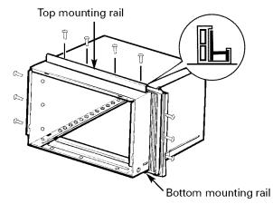
Insert the frames for the accordion panels into the top and bottom mounting rails. Attach the accordion panels to the side of the case using 6 type A screws.
