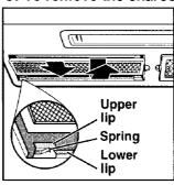
of each filter away from you. This will slide the front of the filter off the lower lip. Swing the front of the filter down and slide the filter out. 6. To replace the grease filters, slide each filter
