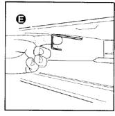
one hand. Pull hook to release microwave hood from mounting plate. If grille cannot be removed (per instructions in pt. 2.), insert a thin looped wire or similar tool through an opening in grille to pull hook.
