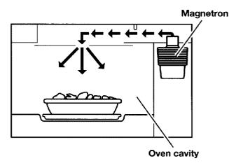
The glass turntable of your microwave oven lets microwaves pass through. Then they bounce off a metal floor, back through the glass turntable, and are absorbed by the food.
