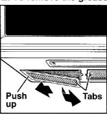
each filter up on the side opposite the tab. Grasp the tab and slide the filter to the side. Pull the filter downward. It will drop out.
