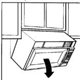
oven downward. (Be careful that door does not swing open.) Lift off the support tabs at the bottom of the mounting plate. Set the microwave oven aside on a protected surface.
