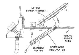
In some areas of the country, spiders or small insects have been known to create "flashback" problems. The spiders spin webs, build nests and lay eggs in the grill's venturi tube(s) obstructing the flow of gas to the burner. The backed-up gas can ignite in the venturi behind the control panel. This is known as a flashback and it can damage your grill and even cause injury.
