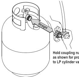
Hold coupling nut and regulator as shown for proper connection to LP cylinder valve.
