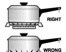
Never extend the flame beyond the outer edge of the utensil. A higher flame simply wastes heat and energy, and increases your risk of being burned by the flame.
