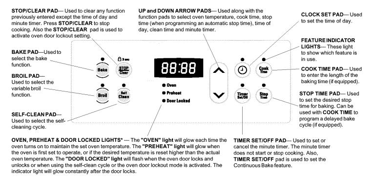
\*Note: The **OVEN** indicator light on the electronic display will turn ON and OFF when using the Bake feature and during preheat. This is normal and indicates that the oven is cycling to maintain the selected baking temperature. When the preheat indicator light turns OFF, your oven is ready.
