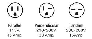
This is recommended for best performance and to prevent overloading house or apartment wiring circuits, which could cause a possible fire hazard from overheating wires. **The 115-volt models** require a 115/120-volt a.c., 60 Hz grounded outlet protected with a 15-amp time delay fuse or circuit breaker.
