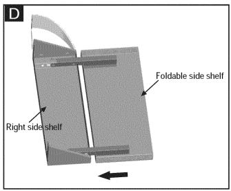
Insert flange on right side shelf into side shelf brackets on side of firebox, shown A.
