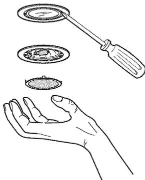
3. Remove the burned out lamp.
