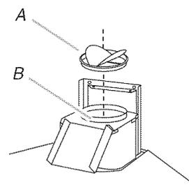
A. Clapet anti-reflux
