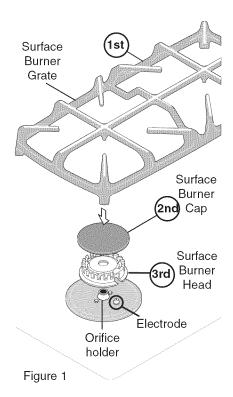
**To Remove and Replace the Surface Burner Caps and Burner Heads -**Remove in the following order: (1st) surface Burner Grates, (2nd) Burner Caps and (3rd) Burner Heads. Replace in the following order: Burner Heads, Burner
