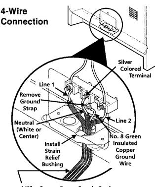
4-Wire Copper Power Supply Cord. To Fused Disconnect Box or Approved Wiring Device for Copper Supply Cord.
