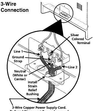
To Fused Disconnect Box or Approved Wiring Device for Copper Supply Cord.
