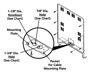
**NOTE:** Range is shipped from factory with 1-3/8" dia. hole as shown. To use either 7/8" dia. hole or 1-1/8" dia. knockouts:
