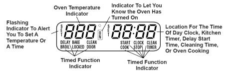
The Control Display is an easy reference for using your oven control. Below are descriptions of how the Control Display works.
