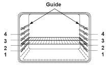
Always place oven racks in the proper position while oven is cool.
