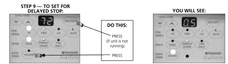
Note: The unit must be running to make this setting.
