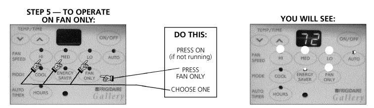
Note: Use this function only when cooling is not desired, such as for room air circulation or to exhaust stale air.(remember to open the vent during this function, but keep it closed during cooling for maximum cooling efficiency.) You can choose any fan speed you prefer. (Note: The "AUTO" setting will not operate in FAN ONLY.)
