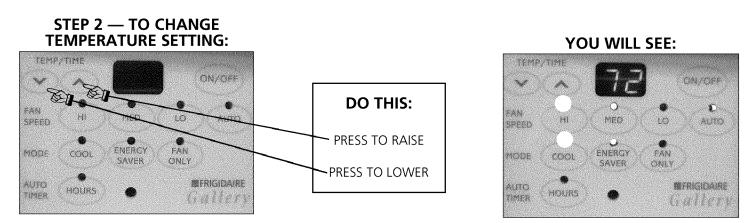
Note: Tap or hold either up( $\land$ ) or down( $\lor$ ) button until the desired temperature is seen on the screen. This temperature will be automatically maintained anywhere between 60F (15C) and 90F (32C). If you want the display to read the actual room temperature, see step 5.
