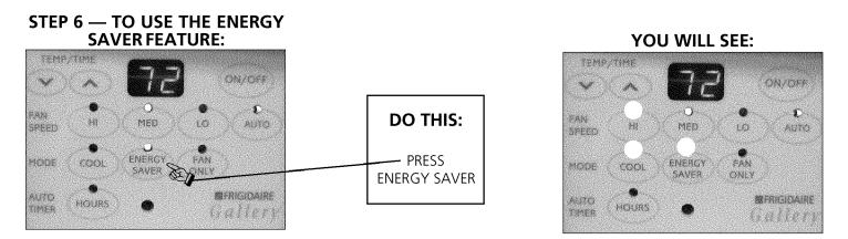
Note: In this mode, when the compressor shuts off, the fan will continue to run for another 3 minutes, then shut off until cooling is needed, as sensed by the room temperature control. During this time, it may come on for 3 minutes to sense whether cooling is needed, then it will go off for 15 minutes. It will continue doing this to sample the room air for as long as necessary.
