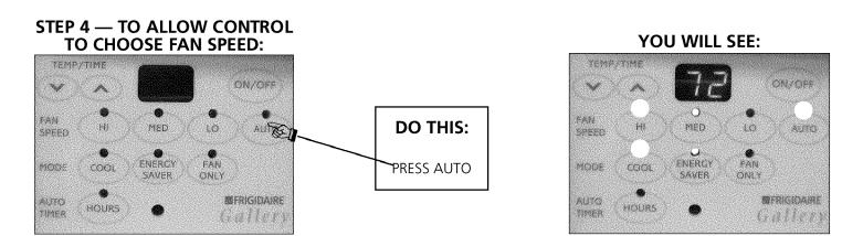
Note: The fan speed will begin in HI, then adjust to MED and LO as the room temperature conditions dictate. For example, if the room doesn't get too warm it will stay at LO. If the room temperature rises quickly, such as a door being opened, it will automatically go to HI speed. The fan speeds will readjust back to LO as the room returns to the original set temperature.
