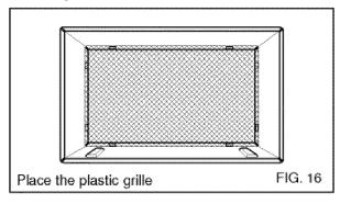
Fasten the 4 washer screws to secure the grille to the wall sleeve. If you need plastic nuts to mount plastic grille to the inside of the wall sleeve, there are plastic nuts in the installation kit. The nuts are installed from the inside of the sleeve and are pressed into the square holes of the rear flanges.
