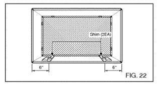
8 Install the new unit into the wall sleeve
