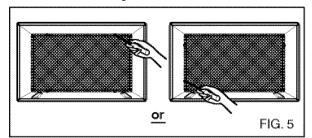
Remove the backing from the Horizontal Insulation strip 13/8 x 3/8 x 273/16 and attach that to the inside bottom of the sleeve as shown below. Remove the backing from the Around Insulation strip  $1\frac{3}{8} \times \frac{3}{4} \times 61^{1/2}$  and attach that to the inside front of the sleeve as shown below.
