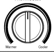
Turn the thermostat control to the desired setting. The central position is a normal setting for average conditions. You can change this setting, if necessary, in accordance with your temperature preference. The thermostat automatically controls cooling or heating, but the fan runs continuously whenever the air conditioner is in operation. If the room is too warm, turn the thermostat control clockwise. If the room is too cool, turn the thermostat control counterclockwise.
