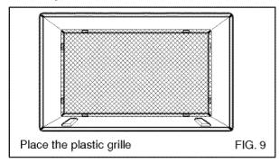
Fasten the 4 washer screws to secure the grille to the wall sleeve. If you need plastic nuts to mount plastic grille to the inside of the wall sleeve, there are plastic nuts in the installation kit. The nuts are installed from the inside of the sleeve and are pressed into the square holes of the rear flanges.
