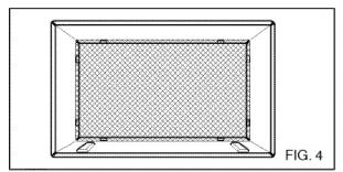
Fasten the 4 washer screws to secure the grille to the wall sleeve. If you need plastic nuts to mount plastic grille to the inside of the wall sleeve, there are plastic nuts in the installation kit. The nuts are installed from the inside of the sleeve and are pressed into the square holes of the rear flanges.
