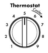
This automatically controls the temperature of the indoor air. Turn the knob so that arrow points to the larger marks for greater cooling. Point the arrow to the smaller marks for more moderate cooling.
