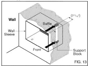
Install the new unit into the wall sleeve.
