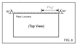
If the wall sleeve already has a rear grille, skip to step 4. If the wall sleeve does not have a rear grille or louvered panel, install the plastic grille from the kit. Cut the plastic grille to 25-1/2" wide and 15-1/4" high. Place the plastic grille to the inside of the wall sleeve at the rear flange.
