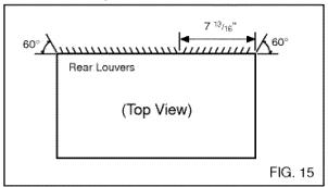
If the wall sleeve already has a rear grille, skip to step 4. If the wall sleeve does not have a rear grille or louvered panel, install the plastic grille from the kit. Cut the plastic grille to 26-1/2" wide and 15-1/2" high. Place the plastic grille to the inside of the wall sleeve at the rear flange.
