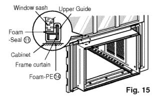
9 Pull each Frame curtain fully to each window sash track, and pull the bottom window sash down behind the Top retainer bar until it meets.
