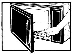
**1.** Empty the microwave oven and clean inside it with a soft, damp cloth. Check for damage such as misaligned door, damage around the door or dents inside the oven or on the exterior. If there is any damage, **do not** operate the unit until it has been checked by an authorized trained service technician and any repair made.
