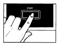
**4.** Push the START Button. The oven light will come on and cooking will begin. You will hear the fan running during oven operation.
