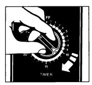
2. Set cooking times up to 25 minutes by turning the Timer Knob clockwise. To reduce the cooking time, turn the Timer Knob counterclockwise. Each mark is 30 seconds for the first 10 minutes. After 10 minutes, each mark is 1 minute.
