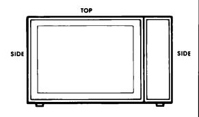
**4.** Do not install the oven next to a conventional surface unit or in any area where excessive heat and steam are generated. This could damage the outside of the cabinet.
