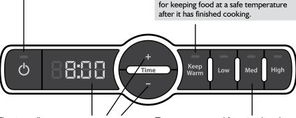
The timer allows you to program a specific cooking time up to 24 hours. By pressing "+" the time will increase by 30 minutes. By pressing "-" the time will decrease by 30 minutes. The time set will be displayed and counted down to zero.
