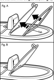
To replace the seal around the edge of the full lid, slowly work the edges of the seal back onto the lid from one end to the other. This seal will fit tightly against both sides of the lip around the bottom of the lid, and will stretch to fit in place.
