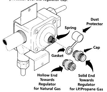
(For Converting Free Standing Ranges from Natural Gas to Liquified Petroleum Gas)
