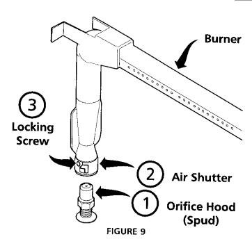
Retest the burner by repeating step "d" above. When the burner flame is a distinct blue color burning steady, the air shutter is adjusted correctly.
