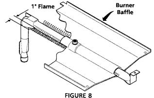
To determine if the oven burner flame is proper:
