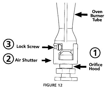
(For Converting Free Standing Ranges from Natural Gas to Liquified Petroleum Gas)
