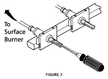
Test to verify if "LOW" setting should be adjusted
