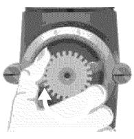
6. When the burrs are touching, turn the grind control gear counterclockwise 1 "click" or detent. The grating or "rubbing" sound will stop. Turn off the mill by flipping the On/Off Switch to the "Off" position. The mill is now calibrated to provide maximum fineness.
