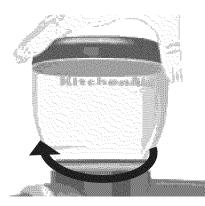
Slide the coffee bin onto the bin platform; the bin seal plate on the motor housing will compress slightly to accommodate the bin. Make certain the bin is centered in the middle of the bin platform.
