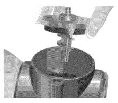
Once the burr-shaft assembly is in the motor housing, rotate the assembly until it falls into place. When correctly positioned, the burrshaft assembly cannot be rotated.
