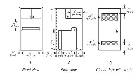
Additional spacing of 1" (2.5 cm) on all sides of the washer is recommended to reduce noise transfer.
