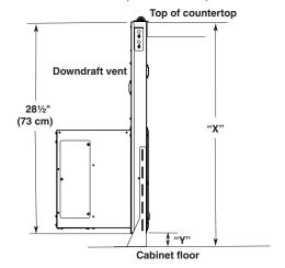
5. Attach the support legs to the side of the vent box with 4 - 4 x 8 mm screws in each support leg. Adjust to dimension "Y" from the bottom of the vent box to the bottom of the support legs. Tighten screws.
