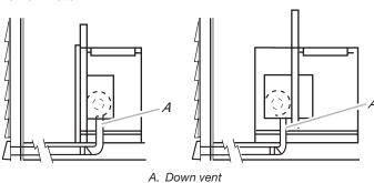
**NOTE:** For island locations, a front- or rear-mounted blower motor can also be mounted for right or left venting if needed for your application. Most island applications would still require the venting to be directed down through the floor.
