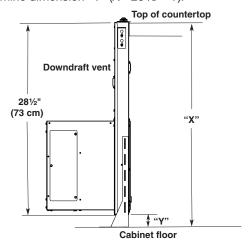
5. Attach the support legs to the side of the vent box with 4 - 4 x 8 mm screws in each support leg. Adjust to dimension "Y" from the bottom of the vent box to the bottom of the support legs. Tighten screws.
