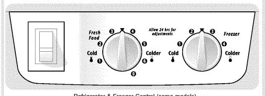
\* **IMPORTANT:** Turning the refrigerator temperature control to "0" turns off the compressor, but does not disconnect the power to the light bulb and other electrical components. To turn off power to your refrigerator, you must unplug the power cord from the wall outlet.
